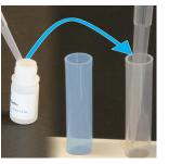
Using a new tip, add 100 μL Buffer to the clear testing tube
