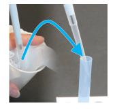
In a separate vessel, dilute extract with water<sup>†</sup> 1:6, for example, 100 μL sample extract to 500 μL water (measure carefully!)
