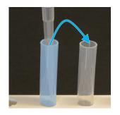
Transfer 100 μL of Step 1's diluted extract from the dilution vessel to the clear tube; stir well with pipette tip
