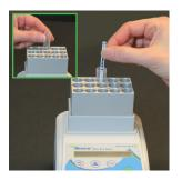
Place tube in Incubator and acclimate for 2 min.\*, then add QuickTox Strip; wait 5 minutes for results
